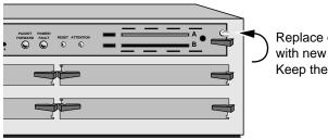
Replace original card in drive A with new copy from drive B. Keep the original card as a backup.
